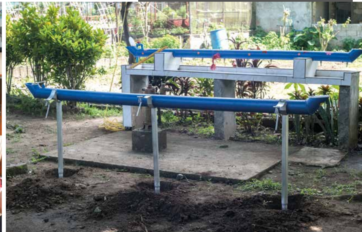
WASHaLOT 3.0 – constructed with a basin and on metal legs // Figure 9
