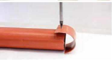
Check the position of part # 3 screwed in part # 5 inside part # 1.
